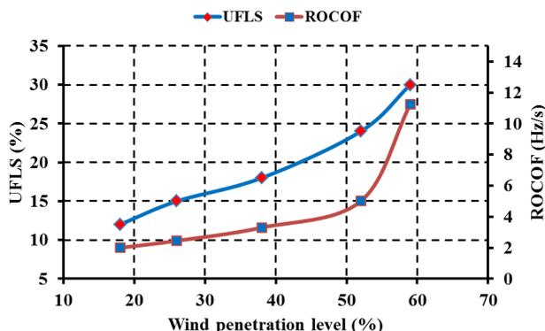
Figure 5. Effects of wind penetration level on UFLS and *ROCOF*
