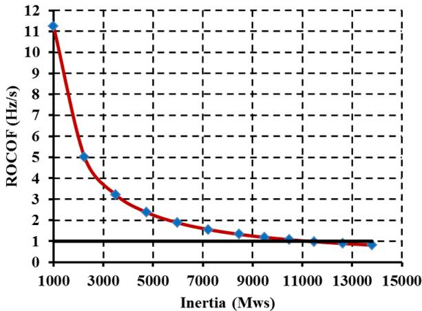
Figure 8. *ROCOF* vs. inertia for single machine case
