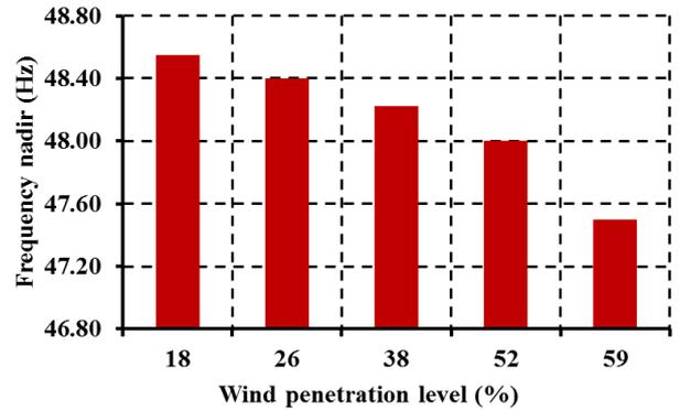
Figure 4. Frequency nadir vs. wind penetration level
